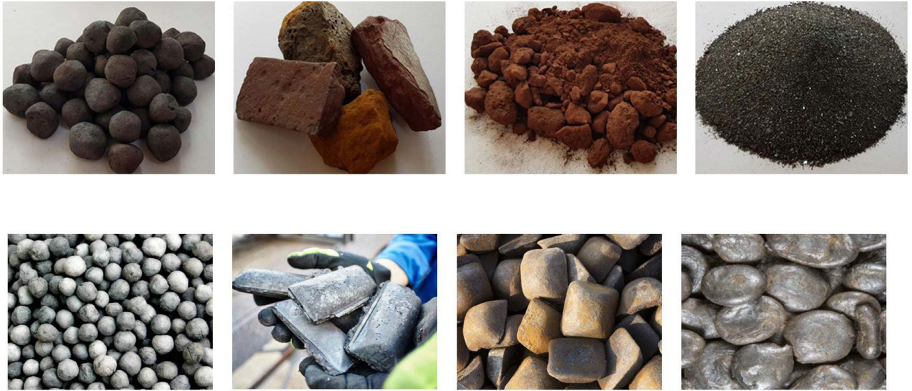
Figure 14: (L-R) top row = ores: DRI pellet, Lump ore, sinter fines (crushed ore), concentrate; (L-R) bottom row = metallics: DRI, HBI, pig iron, GPI
